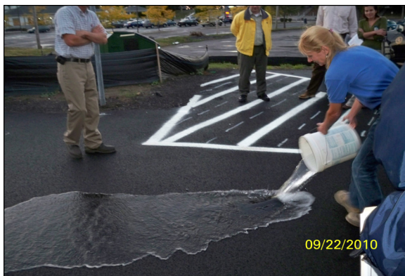
Paula Smith (Monroe County Stormwater Coalition) demonstrating the infiltration capabilities of the porous pavement at Secret Cove Park.
